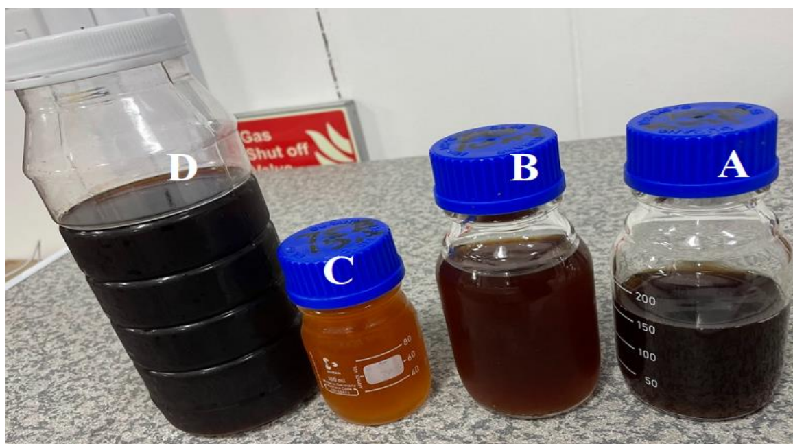
Figure 0.7: The composite of 75%BPE+25%WPE (D), 75%BPE+25%WPE+15 mL ALvE (C), 75%BPE+25%WPE+10 mL ALvE (B), 75%BPE+25%WPE+5 mL ALvE (A).
