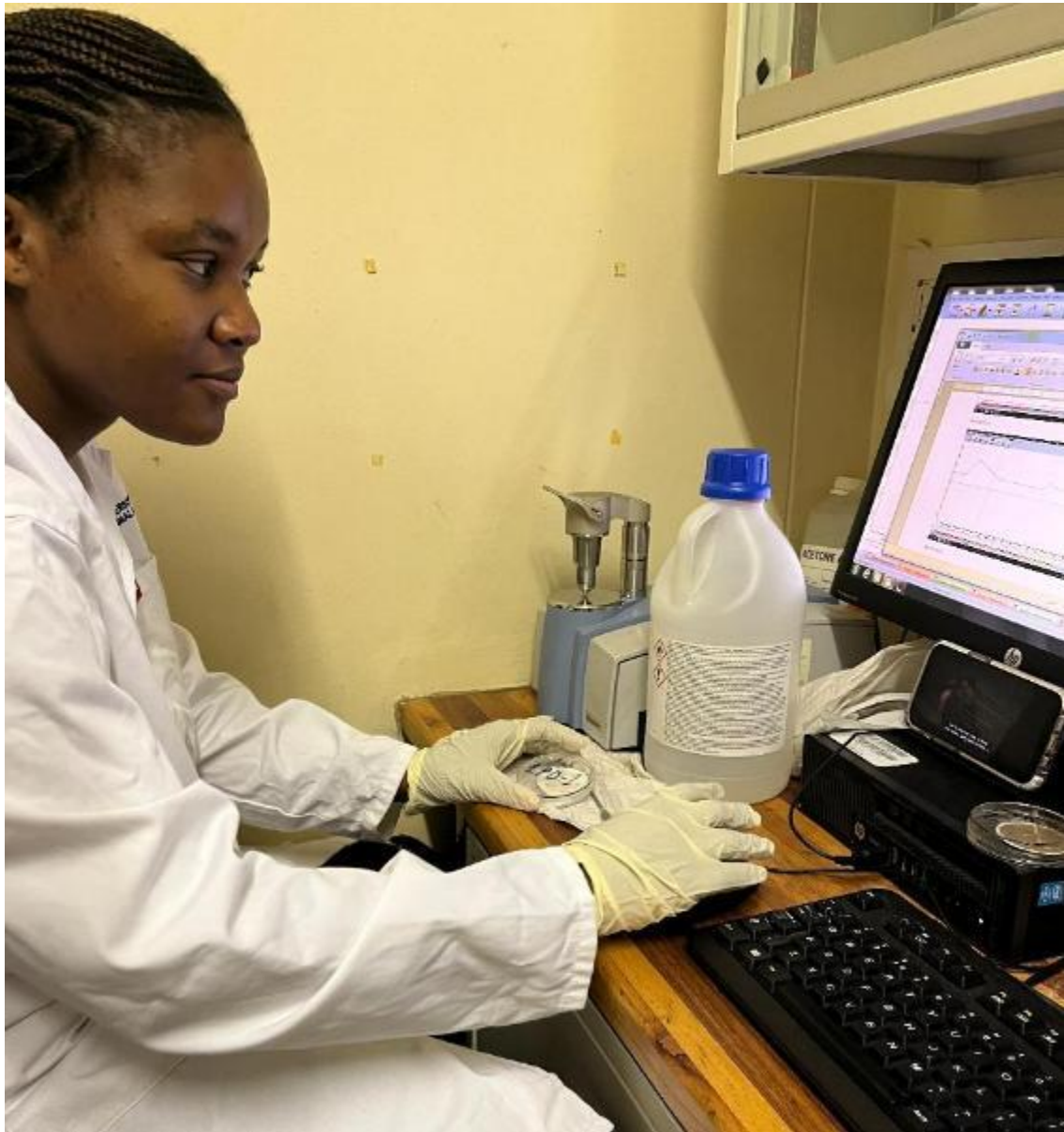
Microplastic polymer identification at the University of Venda using an FTIR spectrometer. Photo by Ayanda Xozmuti
